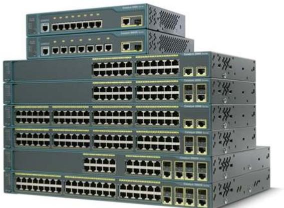
The Cisco Catalyst 2960 LAN Base software image is a rich suite of intelligent services, including advanced QoS, rate limiting, ACLs, and IPv6 management. The SFP-based Gigabit Ethernet ports accommodate a range of SFP transceivers, including the Cisco 1000BASE-SX, 1000BASE-LX, 1000BASE-BX, 1000BASE-ZX, 100BASE-FX, 100BASE-LX, 100BASE-BX, and coarse wavelength-division multiplexing (CWDM) SFP transceivers.
